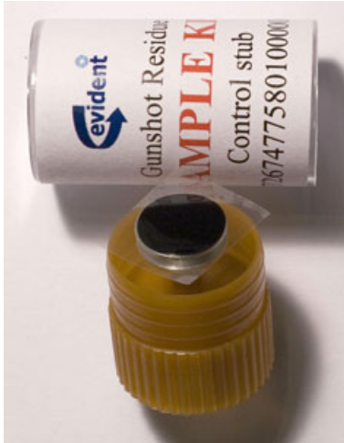
FIG. 1—Example of a stub used for GSR collection.
