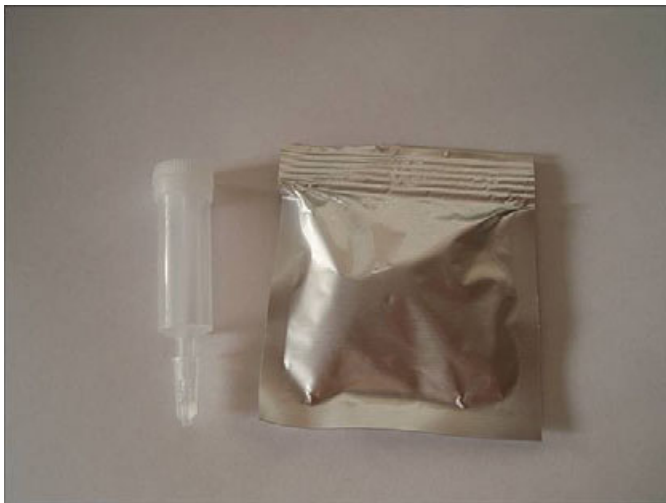
FIG. 2—Example of a swab used for GSR collection.
